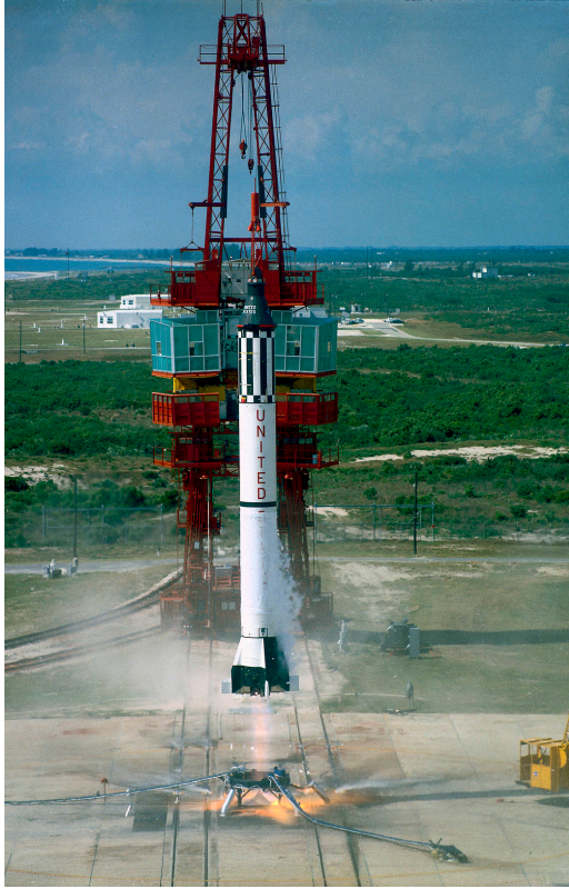
Figure 2. The Redstone launch vehicle
